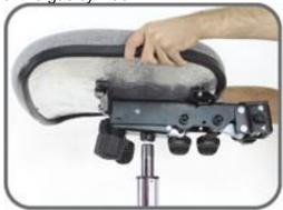
**5.** Remove the knob on the bottom of the seat plate. Reinsert the knob and washers. Tighten.
