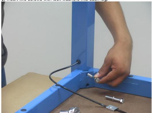
4. Tighten until lock washer is flat. It doesn't have to be tighter than that.
