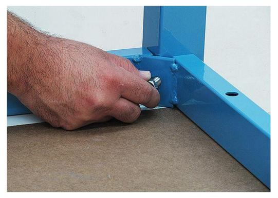
3. Insert a bolt with a lock washer into each leg.
