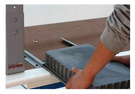
2. Insert three screws on each side. The seventh screw should be positioned near the front as a drawer stop. If you plan to use the drawer to carry product, do not insert the last screw.
