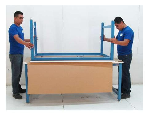
**3.** Insert a bolt with a lock washer into each leg.
