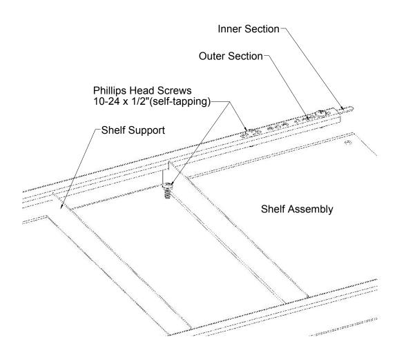
e) Fasten the shelf assembly to the Mounting Brackets with Phillips Head Screws, (10-24 x  $\frac{1}{2}$ ", self-tapping).
